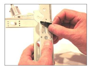
22) Slide the small connector board through the square hole from the inside to the outside. **DO NOT** force it! When oriented correctly, it will slide through the hole without any resistance.
