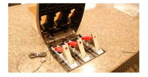
9) Next locate the wires that go to the brake module. Remove the grounding screw (#2 Philips head) that holds the black wire to the pedal assembly.
