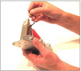
Once you loosen both screws, if they continue to rotate and not come out, try putting pressure on the pedal face while turning the screws.
