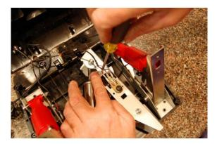
37) Place the Perfect Pedal module in place on the base. Holding the black cover up at a 90 degree angle, clip the wiring harness back into position and make sure the wire exiting the pedal assembly is in the provided notch.
