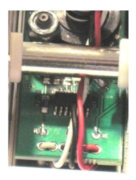
**CAUTION:** If the wires are not run behind the bolt they can become pinched under the pedal face and be damaged. This damage and any subsequent damage caused to the computer or the Perfect Pedal electronics **WILL NOT** be covered by the warranty.
