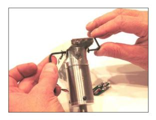
33) Install the shoulder bolt through the pedal base, holding the shaft of the Perfect Pedal in place. Make sure that you position the two spacers, one on each side of the shaft. The spacers in your kit may be either black or silver.
