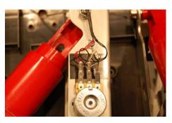
10) Take needle-nose-pliers and carefully remove the 3 spade connectors, one at a time from the brake module. Remove the brake module.
