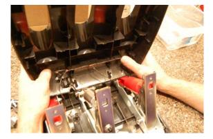
38) Replace the top cover and invert the pedal assembly holding it together until you insert and tighten the two silver screws in the upper corners of the pedal assembly.
