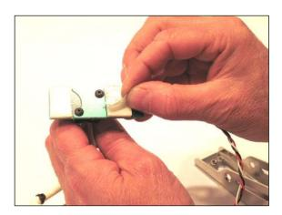
20) Align the end of the circuit board where the wires exit, flush with the bottom of the pedal face and press firmly in place.
