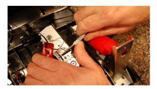
11) Using a 2.5 mm allen wrench, remove the two screws that hold the red plastic piston to the pedal face.
