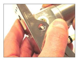
32) Using two 2.5 mm Allen wrenches tighten the screws making sure that BOTH SIDES are tight.
