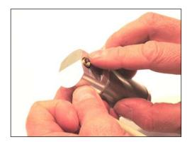
**NOTE:** If the hole that the brass shaft fits into on your Perfect Pedal cylinder has a black bushing in it, there is no need to grease the shaft. Your kit may or may not have a supplied grease packet.
