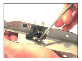
15) Slide the black plastic gear and spring off the potentiometer.
