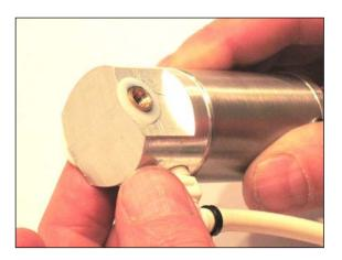
31) Align the cylinder so that you can see the end of the brass shafts' threaded holes through the hole in the pedal face and start the screws with your fingers.
