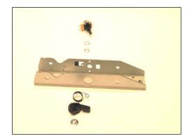
17) Loosen the Philips Head Screw that retains the black plastic gear on the pedal face and remove it.
