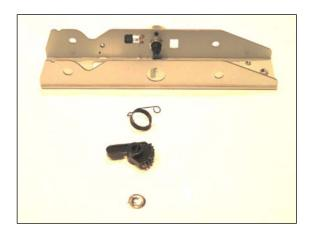
16) Remove the 11 mm nut holding the potentiometer to the pedal base then remove the potentiometer and spring.
