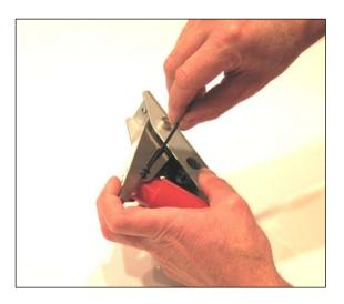
12) Remove and save the brass shaft from the red plastic piston.
