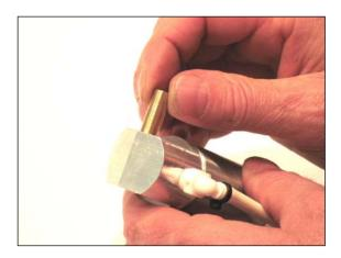
**NOTE:** <u>DO NOT</u> force it. It should drop through the hole freely with no resistance. In some rare cases (pedals with very high hours) the ends of the brass shaft may have burrs on it. If the brass shaft will not slide freely in the hole in the cylinder you must remove any burrs on the ends of the brass shaft using a file or fine sandpaper.
