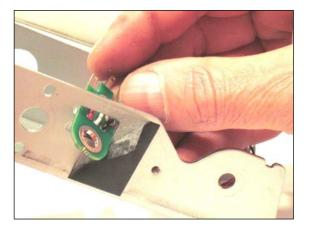
23) Smooth the black tape back onto the pedal base.
