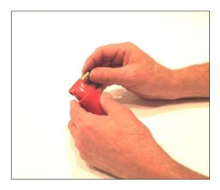
13) Remove both shoulder bolts that hold the base of the plastic piston and the pedal face to the pedal frame.
