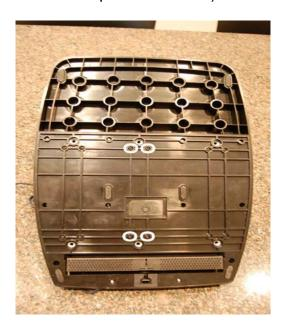
6) Next remove the 14 silver screws including the 2 screws under the carpet bar. (These are #1 Phillips head screws.)
