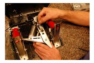
36) Next, screw the grounding screw and black wire back in place. Make sure the wire end is pointing towards the top of the Perfect Pedal module.
