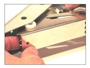
27) Install the shoulder bolt that holds the pedal face in the pedal base making sure that the wires run behind the shoulder bolt.
