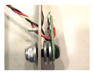
25) Tighten the bolt so the connectors face towards the back of the pedal base.
